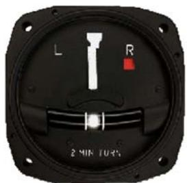
The 9500 Series Turn and Slip Indicators have been designed with emphasis on safety and reliability. Conventional restraining coil springs have been replaced by a single spiral torsion spring secured at the gimbal shaft. A patented viscous fluid device on the gimbal shaft dampens the gyro response to applied forces. Use of the "Hall Effect" brushless
