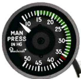
The Manifold Pressure Indicator is used on aircraft to indicate the absolute pressure of the aircraft engine intake manifold in Inches of Mercury Absolute.
