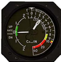
The Indicator is a triple function unit displaying three indications. The inner scale displays the pressure inside the cabin in feet of altitude. The upper right side scale displays the difference in pressure between the inside and the outside of the cabin in pounds per square inch. The left side scale displays the rate of climb in feet per minute ascent or descent.
