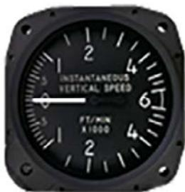
The 7100 Series Instantaneous Vertical Speed Indicator is a precision instrument, which provides an accurate and reliable indication of rate of change of altitude. Ascent is indicated by a clockwise rotation of the pointer from zero. Descent is indicated by a counter clockwise rotation. Zero is at the 9 o'clock position. Stops limit pointer movement at the end of the scale. A zero adjustment screw is located on the face of the case at the seven o'clock position.
