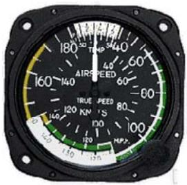
The 8100 Series True Airspeed Indicator is intended for use on an aircraft to indicate the speed relative to the air at sea level or the desired altitude, to indicate the equivalent speed corresponding to the actual force of the air. The indicator has an inner dial to indicate true airspeed. That is, the altitude and temperature are the conversion factors used to obtain this reading with the use of a setting knob.
