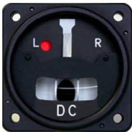
The 9500 Series Turn and Slip Indicators have been designed with emphasis on safety and reliability. Conventional restraining coil springs have been replaced by a single spiral torsion spring secured at the gimbal shaft. A patented viscous fluid device on the gimbal shaft dampens the gyro response to applied forces. Use of the "Hall Effect" brushless DC gyro motor
