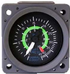
The Indicator is a dual function unit displaying two pressure indications from two independent mechanisms. The outer scale displays the pressure inside the cabin in feet of altitude. The inner scale displays the difference in pressure between the inside and the outside of the cabin in pounds per square inch (PSI).
