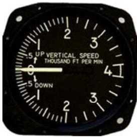
The 7000 Series Vertical Speed Indicator is a precision instrument, which provides an accurate and reliable indication of rate of change of altitude. Ascent is indicated by a clockwise rotation of the pointer from zero. Descent is indicated by a counter clockwise rotation. Zero is at the 9 o'clock position. Stops limit pointer movement at the end of the scale. A zero adjustment screw is located on the face of the case at the seven o'clock position.
